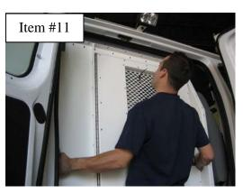
Place the **3<sup>rd</sup> Compartment Doorframe** assembly.
